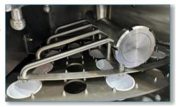
Additionally the machine features a cup leakage test function that detects any leaks from the membrane lid, the seal or the cups. In the event of a defective package, the machines built-in function for disposal removes it, thereby further enhancing the safety and reliability of your production line.
