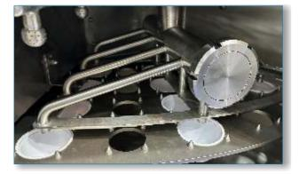
Additionally the machine features a cup leakage test function that detects any leaks from the membrane lid, the seal or the cups. In the event of a defective package, the machines built-in function for disposal removes it, thereby further enhancing the safety and reliability of your production line.
